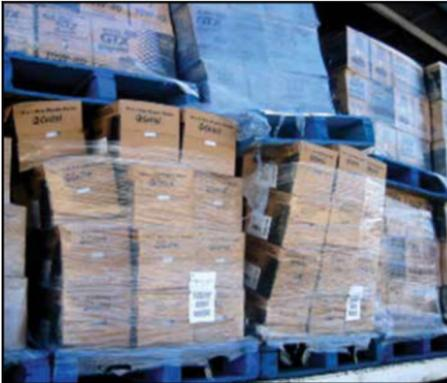
*Example of the type of load that requires adequate and suitable securing.*
