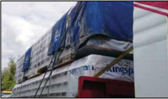
*This load is shown with additional securing. An additional hammock strap and cross-strap was fitted after the vehicle had been stopped at roadside. This arrangement was adequate to restrain a load of this weight and to allow the truck to carry on.*
