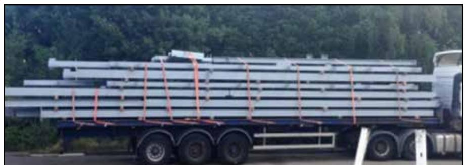
Examples of loads above the headboard which require additional securing, more than is shown in the pictures. Additional lashing is required – both top-over lashing to increase downward loading plus additional lashing/support across the front of the load to prevent forward movement, possibly a temporary headboard or heavy-duty hammock/sail sheet.
