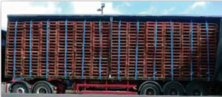
*A light load with a difference. None of the pallet stacks exceed c.400kg, so internal straps are appropriate.*
