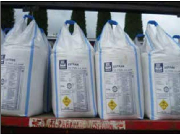
*Not secured in a curtainsider – unacceptable.*
