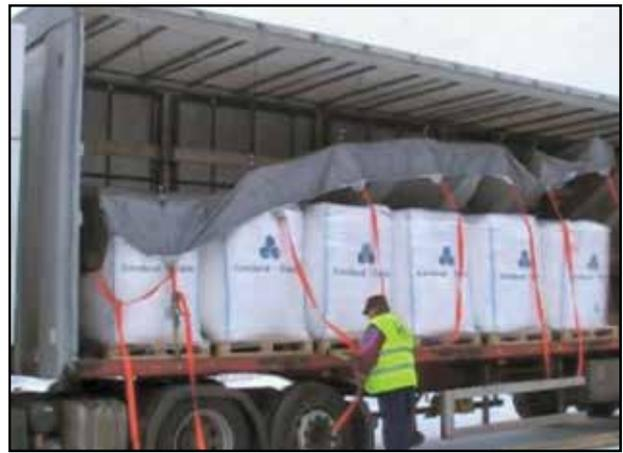
*A suitable alternative system for load-securing.*
